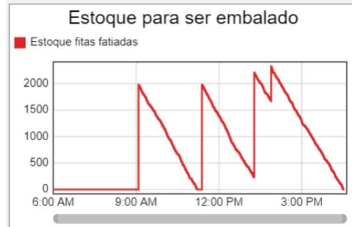
**Figure 14.** Intermediate Stock per machine - standard scenario
